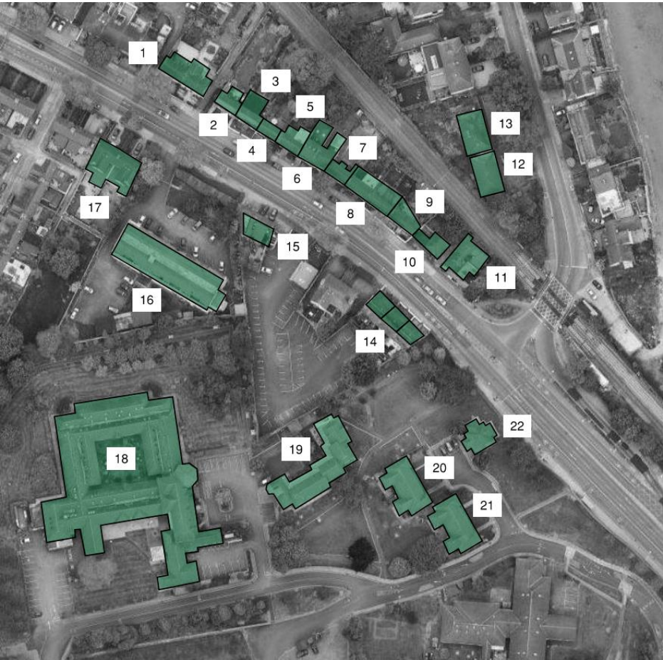
Figure 2 – A graphic showing the properties assessed. Green denotes that results sit inside of the BR 209 (2022) recommendations. The numbers correspond to the list of property names given below.
