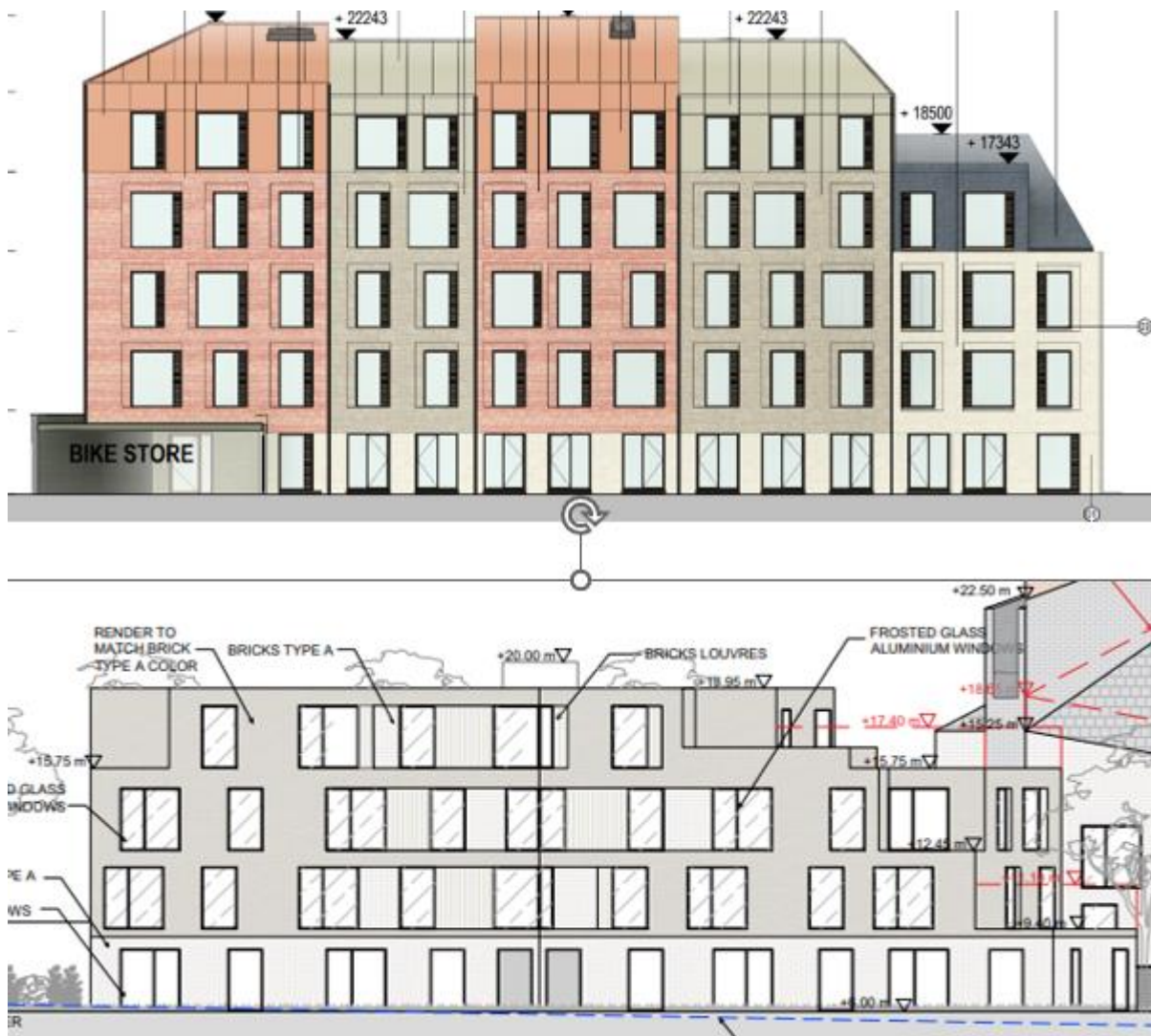
Figure 15 Block B South East Elevation - proposed on top, permitted below
